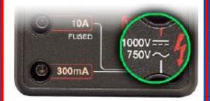
Do not use meters without proper CAT markings on 480 V circuits
